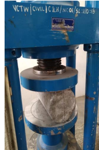
Figure.5 Testing of split tensile strength
