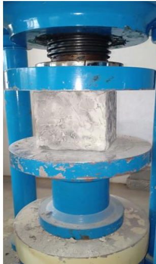
Figure.3 Testing of compressive strength
